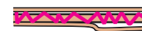
Forbidden route drawn irregularly, gives appearance of crossing points. Obscures adjacent permitted route
